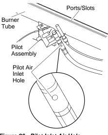
Figure 26 - Pilot Inlet Air Hole
